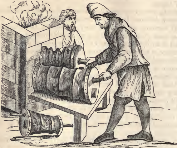
No. 105. Lantern Bellows from Agricola
